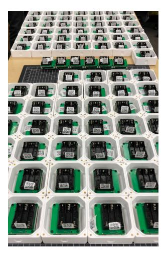
In the end, Additive at Scale designed an electronic enclosure complete with an O-ring groove and seal, threaded inserts, and custom PCB mounts, and printed 100 units for their pilot phase with an Essentium HSE 180 ST 3D Printer.
