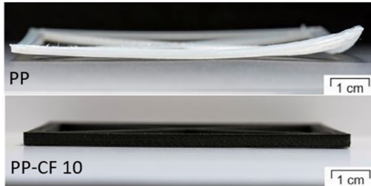
Figure 9: Warpage/Curling behavior in PP vs PP-CF 10 [3]
