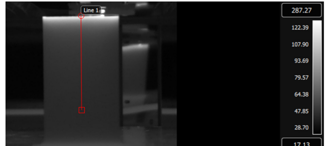
Figure 7: Temperature gradient in a section of HTN-CF25 plaque along the Z-direction. The image was recorded using an infrared camera system during the printing process. Line 1 shown here denotes where data is collected. The temperature scale is shown to the right, with a maximum temperature of 287.27 °C and a minimum temperature of 17.13 °C.
